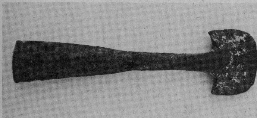
The Bark Spud—Used on the end of a long handle to strip oak bark from trees.
