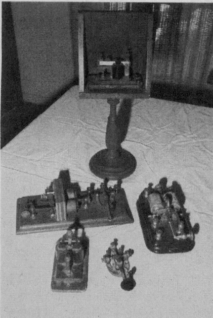
Telegraphy equipment donated by W. K. Baker to the Gunnison Museum includes (from top, clockwise), sounder, relay, key, sounder and key with sounder.
