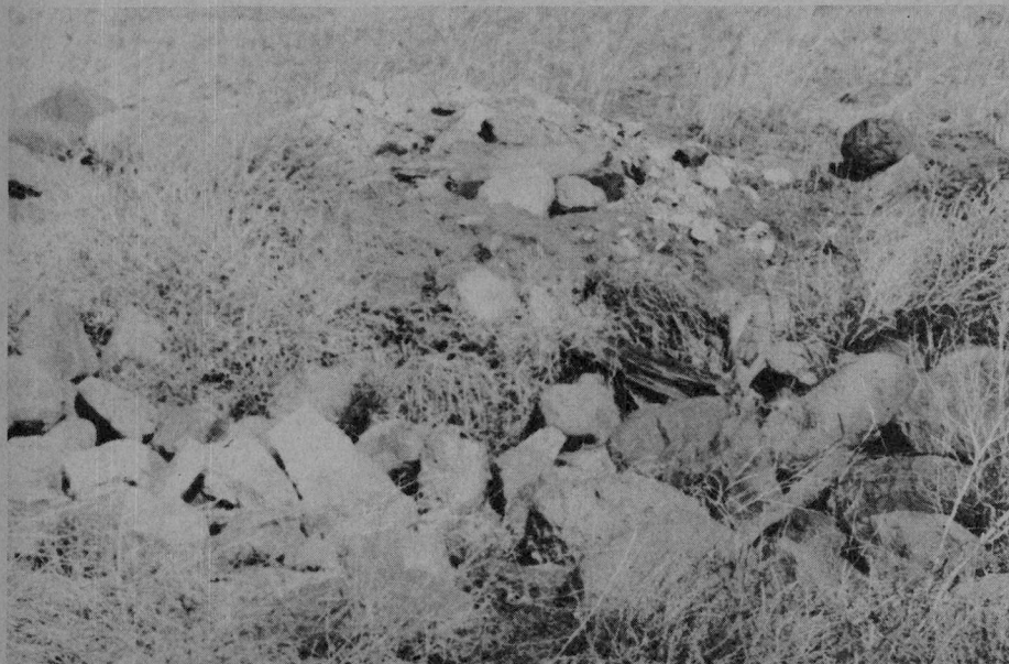
Old mine shafts were usually filled in with rock and rubble.
