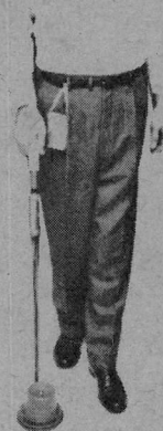
The COIN-RANGER in action. The "Companion Receiving Unit" containing the loud-speaker is shown clipped to operator's belt.
