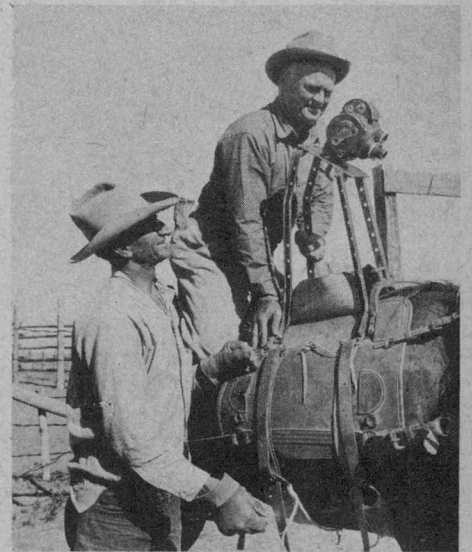
Details of special camera mount we used with an automatic camera to get a bronc rider's view of bucking action. Results? One big blur!
