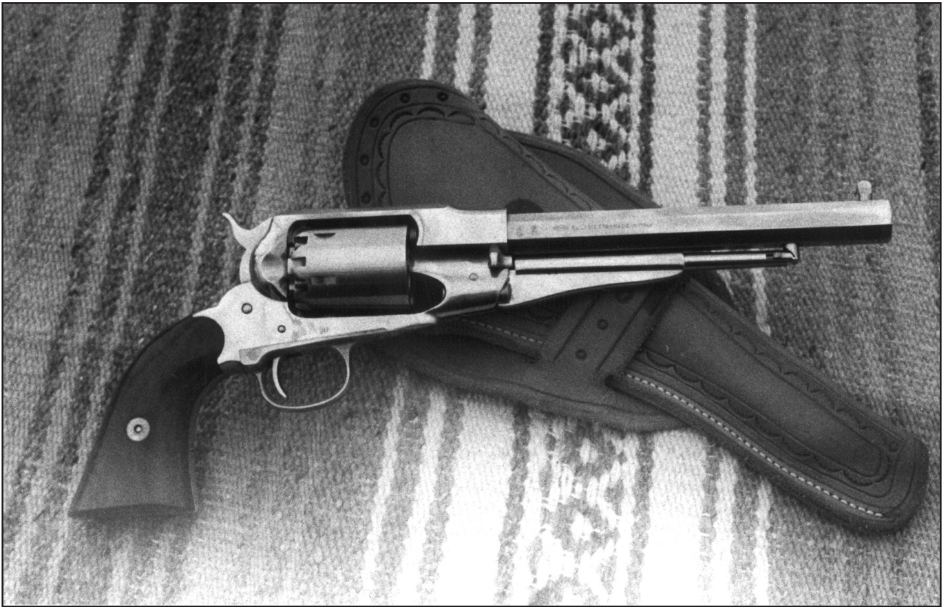
A modern replica of a Model 1858 percussion Remington revolver. This model is popular for competitive shooting. Author's Collection.
