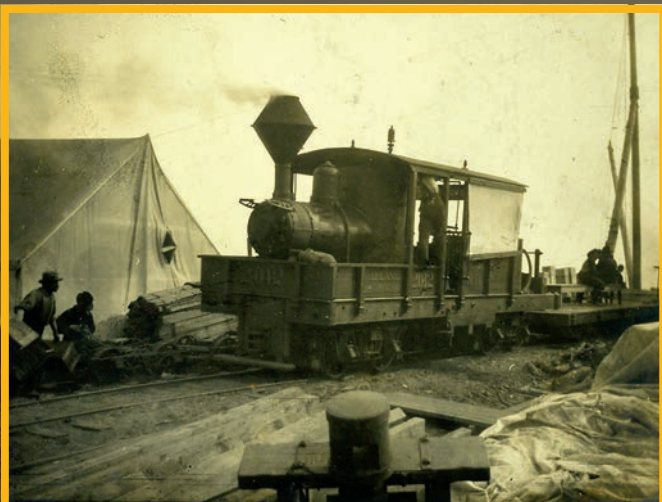
In July 1900, four miles of the Wild Goose Railroad opened from Nome to the Anvil Creek mining district. This is most likely the narrow-gauge's Climax Class A locomotive near its railhead in Nome.
